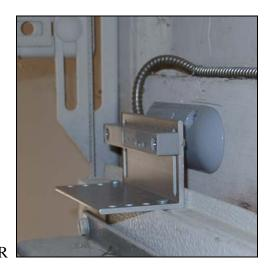
Attach the **non-wired Sensor Completer** to the interior side of the garage door in one of two places:
